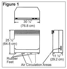
**restrict air circulation**. If installing the fireplace in a carpeted area, place a onepiece, solid, flat surface under the fireplace insert. Ensure that all four of the insert's feet rest securely on this surface.
